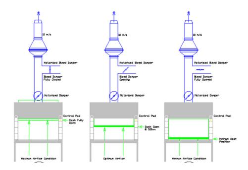
This initial volume is calculated as being the volume through the fume cupboard at a sash opening of 0.5m at a velocity of 0.5m/sec by the internal width of the fume cupboard. I.e. 0.5x0.5x internal width of the fume cupboard. The minimum volume, therefore, is 0.33x0.5x0.5 internal width of the fume cupboard.
